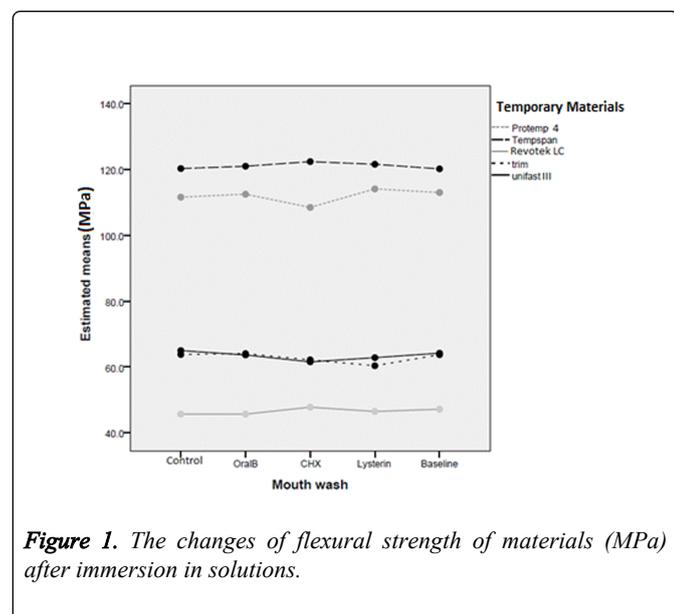
**Figure 1.** The changes of flexural strength of materials (MPa) after immersion in solutions.
