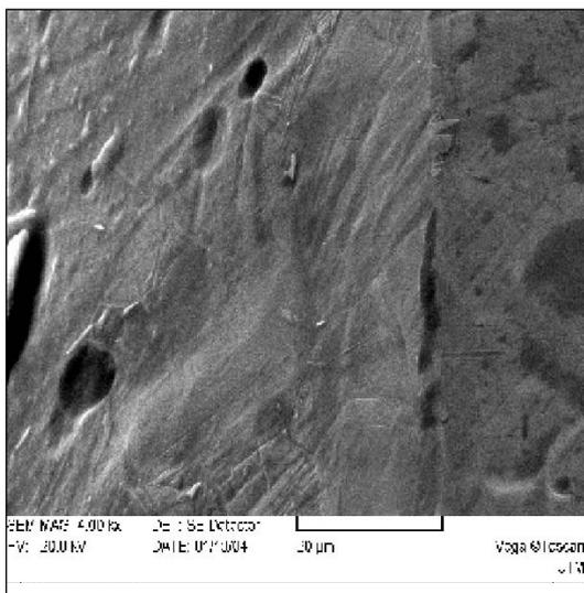
Figure 1. Unprocessed Ti surface
