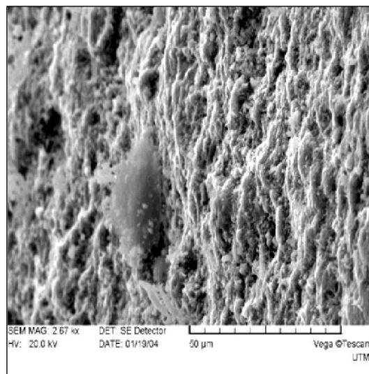
Figure 2. Surface processed by anode oxidation
